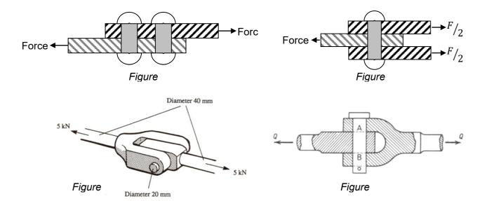
Discuss and compare the advantages and limitations of single shear (Figure A) and double shear riveted joints (Figures B, C, D and E). Within your discussion compare and contrast joints using single and double shear arrangements in addition to using typical worked numerical examples to validate key areas of your discussion.
